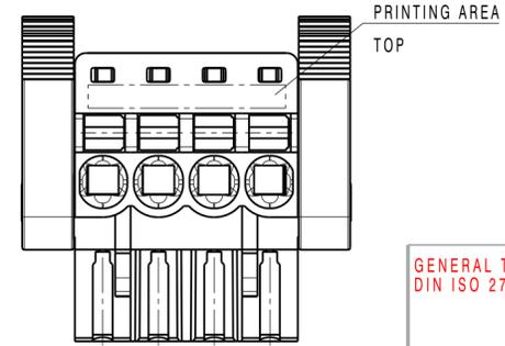
For the mounting of PCBs, it should be noted that the rated data relates only to the PCB components alone. The necessary creepage and clearance paths must be observed in connection with the respective applicant in accordance to IEC 664 / VDE 0110. The current-carrying capacity and pitch tolerance is to be determined according to DIN IEC 326 part 3 very fine.
