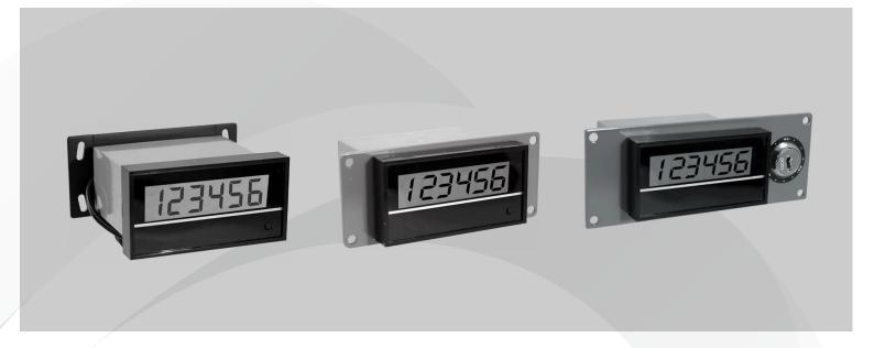
A 6 figure, battery powered, push-button or key reset, electronic counter, available in base mount or panel mount configuration. No external power supply is required. Large 0.50" [12mm] LCD figures for fast, easy reading. Operates at 6-240 VAC or VDC. Long lasting internal lithium battery. Attractive styling and silent operation make these models equally well-suited for lab or office equipment applications.
